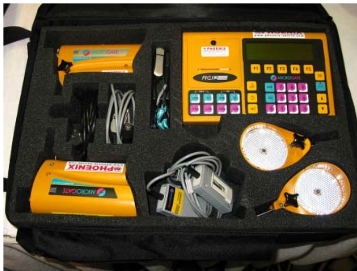
Note the antenna on top of the finish line sensor. There are no wires. The whole system fits into two suitcases.
