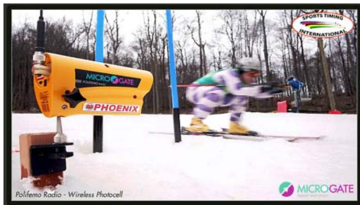
Note the antenna on top of the finish line sensor. There are no wires. The whole system fits into two suitcases.
